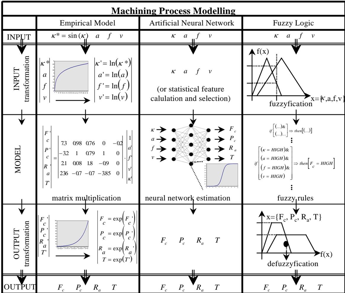
Figure 3. Data handling of three cutting model methods
