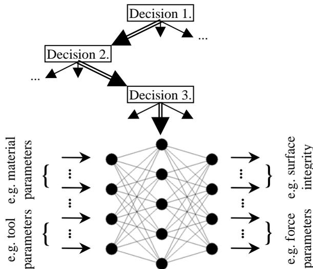
Figure 5. The use of the ANN based cutting model.
